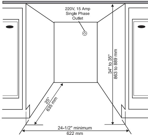
ASKO dryers can be installed beneath a cabinet or worktop with a minimum height of 34" (864 mm). There must be a gap of about 1/2" (12 mm) all around the machine and a minimum gap of 1" (25 mm) between the rear edge of the machine top panel and the back wall. The opening width must be at least 24-1/2" (622 mm). The condensing models work best when they have good air circulation.
