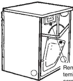
Remove cover to access terminal box. (Requires- Torx screwdriver.)
