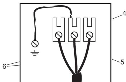
5. Connect ground (center) wire of power supply cord to the center, silver-colored terminal screw. Tighten screw.
