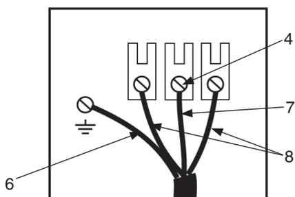
5. Remove ground wire (green with yellow stripes) from external ground connector screw and remove from center terminal block.
